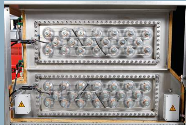
Installation example of a tank with plate type transducers - exterior view
