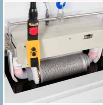
Electrolytic polishing of small parts as bulk material in drums
