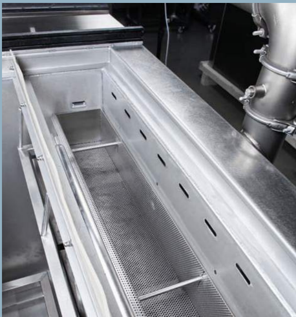
Overflow pocket, coarse filter and integrated exhausting
