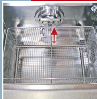
KTRO: Unit with basket oscillation
