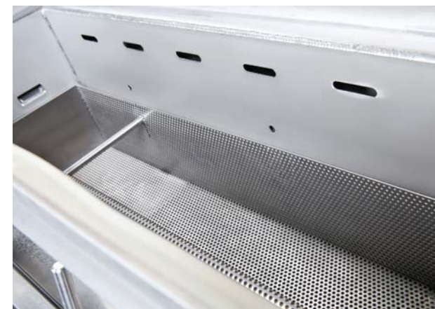
Overflow pocket, coarse filter and integrated exhausting
